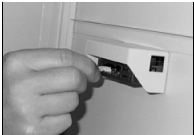
Fig. 29: Disconnect the connector from the display
